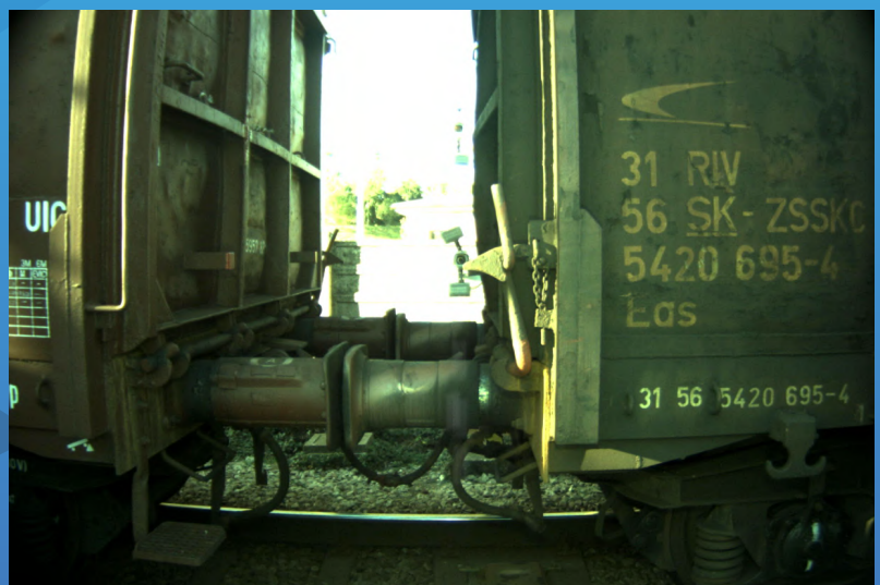
Right: an image of a UIC code of a railway wagon acquired by a side camera.
